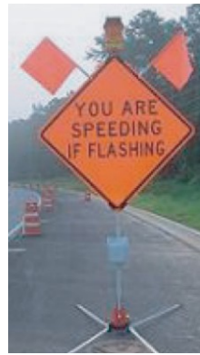
Source: Mattox, et al. Development and evaluation of speed-activated sign to reduce speeds in work zones.
